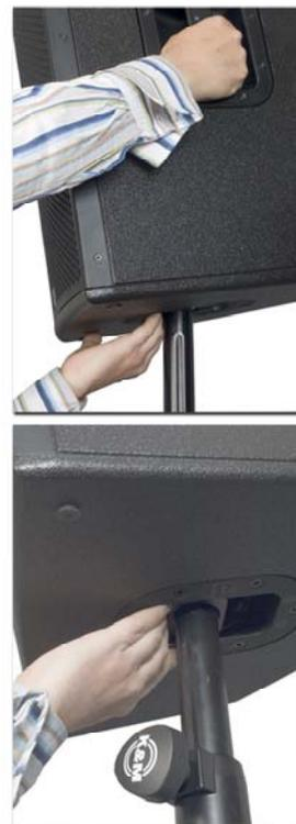
Please lift up the loudspeaker slightly and justify it in the right declination as shown on page 20. When lifting up the speaker too hard it can be removed from the high stand. If you set down the box on the high stand, the flange must snap in.
